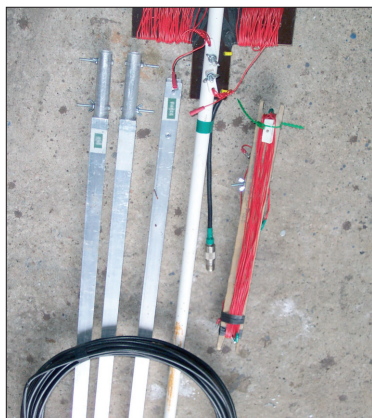
Fig. 6: Three 1.52m lengths with a round section riveted into one end. These all slot together making a 4.6m free standing mast (see text).
