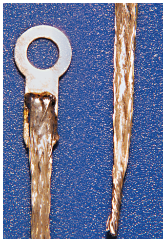
● Fig. 1: The ends of an earth-strap made from the otherwise discarded screen of coaxial cable.
