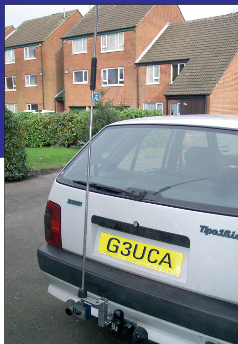
Fig. 2: The decision to fit the bracket using the bolts - which hold the tow ball to the tow bracket - was taken by G3UCA as this would provide a very good earth to the car body (see text).
