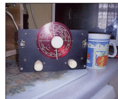
● Fig. 3a, b, c: Different views of three-valve EF50 design built by G4JCP's e-mail 'keyboard-pal' Wally Bell. The set is really quite small and very attractive. Inside, it's very reminiscent of an American midget receiver.
