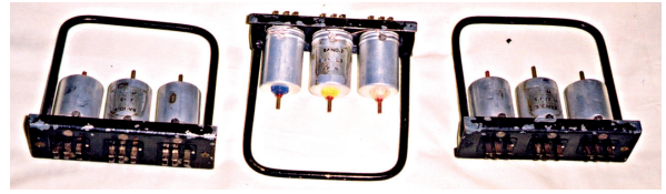
● Fig. 3: The Denco coil units for the 1963 receiver were mounted as plug-in units (see text).
